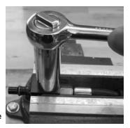
Use the o-ring removal tool to remove the oring.
