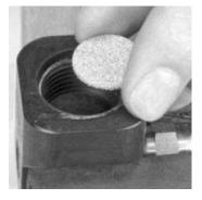
4. Screw the Quick-Fill adapter into the manifold by hand.
