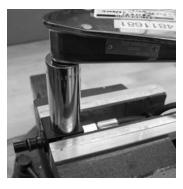
**NOTE:** Applying light downward pressure to the head of the torque wrench with your free hand during installation will better secure the socket to the Snap-Tite aluminum plug.
