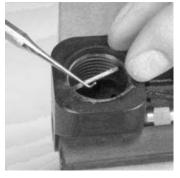
4. Use the o-ring removal tool to remove the oring.
